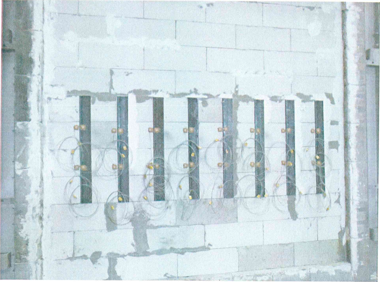
Photo C1: Unexposed side of the test construction before the test
